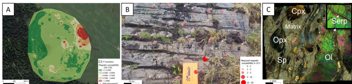
Figure 1: Different scales of serpentinization heterogeneity A) Magnetic susceptibility map of the whole peridotite body, high values are located to the north-east; B) Magnetic susceptibility of a meter-size block, where highest values are located along the fracture network; C) Thin section of the TT lherzolite. Opx: Orthopyroxene, Cpx: Clinopyroxene, Ol: Olivine, Sp: Spinel, Matrix: Minerals in fine-grained matrix, Serpentine (Serp) in mesh structure olivine.
